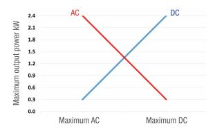
The total output power per module is 2.7 kW, limited to 2.4 kW for each AC or DC port.
